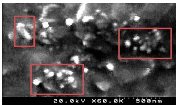
Figure 4. SEM micrographs of epoxy nanocomposites containing MWCNT and \text{Fe}_2\text{O}_3 hybrid nanofillers. [Color figure can be viewed in the online issue, which is available at wileyonlinelibrary.com .]
